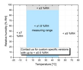
Fig. 1: Typical tolerance of the % RH measurement
